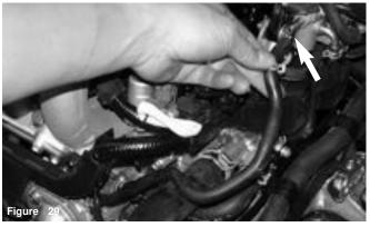
The stock hose is pressed over the upper intake manifold port as shown above.
