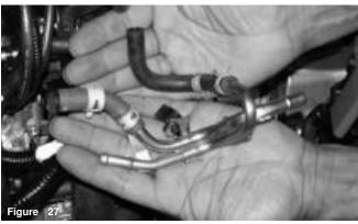
All lines have been removed or disconnected and the PCV  $\,$  hard line is now ready  $\,$  to be removed.
