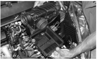
The remaining air box is now pulled from the engine compartment.
