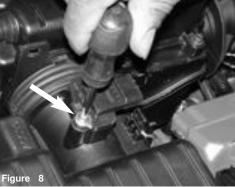
Loosen and removed the two bolts that fastens the mass air flow sensor in place.
