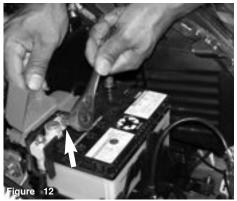
The negative and positive battery terminals are loosened and removed.
