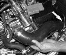
The silicone intake is inserted into the front bumper opening.
