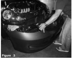
Remove lower screws by the wheel well and the remaining plastic retaining clips Once the plastic clips and screws have been removed, continue to slide the bumper off.
