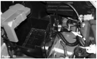
Loosen and remove the m6 bolt that holds the battery case to the frame. The extended bracket is located behind the head lamp.
