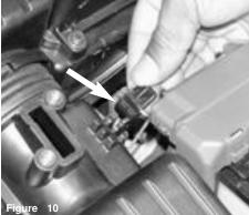
Remove the plastic clip on wire hinges located on the sensor housing facing the driver side.
