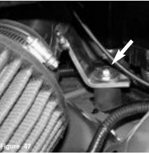
The m6 flange nut and fender washer is tightened over the vibra-mount stud.
