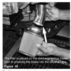
The filter is inserted into the end of the intake. Once the filter stops butt up against the intake, continue to tighten the filter neck clamp.
