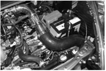
Align the entire intake for the best possible fit. Once the intake has been cleared from all moving parts, continue to tighten all nuts, bolts and clamps. Periodically, check the fitment of the entire intake to prevent damage to the intake.
