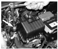
Loosen and remove the first bolt from the air box cleaner.
