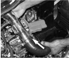
The silicone intake is pressed over the end of the
