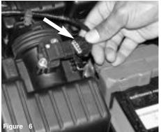
Remove the electrical harness clip from the mass air sensor.
