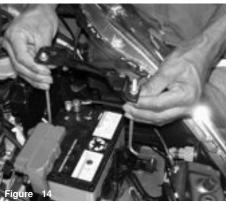
once you have unhooked the tie down rods, the entire tie down is removed.
