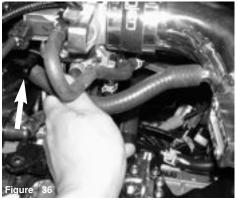
The other end of the 10mm hose is pressed over the crankcase vacuum port.
