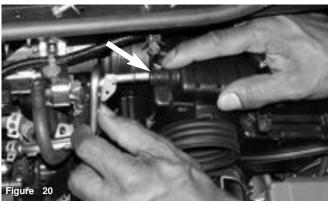
The PCV vacuum hard line is pulled from the air box port.
