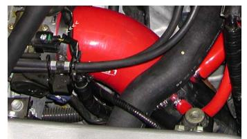
Press the 2 7/8" end of the molded elbow over the throttle body. Position the elbow downward and semi-tighten one of the clamps on the elbow.
