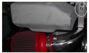
Align the straight bracket on the intake to the vibra-mount stud, use the m6 flange nut and fender washer to secure the intake in place (A). Press the filter over the end of the intake and tighten the clamp located on the filter neck (B).
