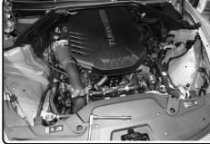
**11.** Both stock intakes removed from vehicles.
