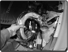
**15.** Install the Driver side tube and position the bracket to the vibramount and turbo. Do not tighten.
