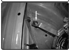
**20.** Secure the bracket on passenger side using provided fender washer and nut. Position intake for the best fit and tighten clamps using 8mm nut driver.
