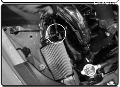
**21.** Install the air filter to the passenger side and tighten using 8mm nut driver. Readjust if necessary for best fit.
