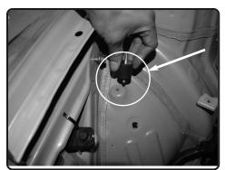
**12.** Install the provided vibramount to the original air box mounting insert on passenger side. Secure and tighten.
