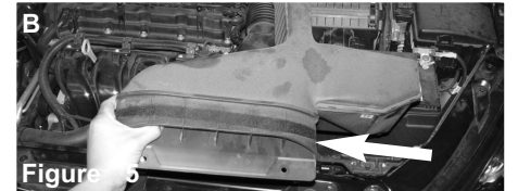
Figure 5 Figure A: Use a phillips screw driver and remove the two plastic retaining screws on the front vent duct. Figure B: This air duct will be removed.
