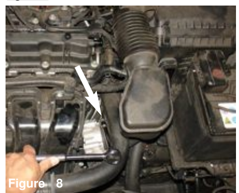
Figure 5 Figure A: Use a phillips screw driver and remove the two plastic retaining screws on the front vent duct. Figure B: This air duct will be removed.
