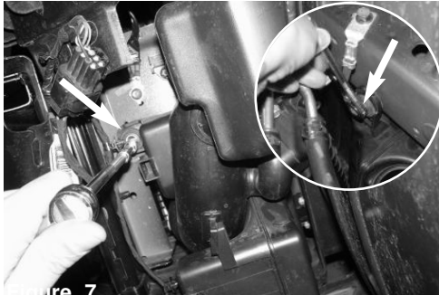
Figure 7 Locate the air box resonator located in the drivers side bumper cavity. Remove the two 10mm bolts attaching it to the chassis. One bolt is located in the engine bay
