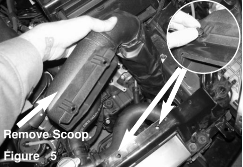
Figure 5 Remove the 2 push clips from the front of the radiator support holding in the ram scoop and then remove the air scoop.
