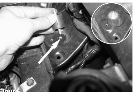
Figure 9 Install the vibra mount to threaded insert on the chassis in the engine bay behind the drivers side headlight. Secure the vibra mount and tighten.
