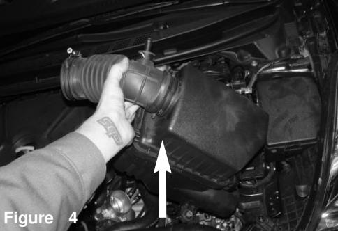
Figure 4 Now lift up and remove the stock intake assembly from the vehicle.
