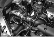
Place the 2.875" hose and two clamps onto the turbo inlet Use two supplied M4 screws and secure the MAF sensor to the intake pipe using a 2.5mm allen.
