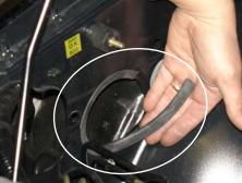
Use the 12" vinyl flex trim to align the resonator opening. The entire resonator opening must be covered to prevent the edge from cutting into the intake.
