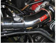
Take the primary intake and press the 3" end into the inlet hose as shown above. The clamp is semitightened to hold the intake in place.
