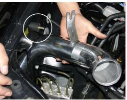
Insert the secondary intake in the resonator opening and
