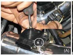
Use the stock screws to fasten down the mass air flow sensor (A), continue to press harness clip over MAF sensor until you hear it snap in place (B). Page 2 of part# SP1202
