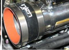
Press the 2 3/4" straight hose over the end of the primary intake. Use two .312 Power-bands and tighten the clamp located on the intake side (A).
