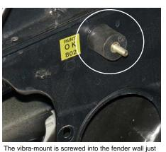
above the round resonator opening. The vibramount is screwed in until it bottoms out.
