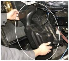
This installation will require the removal of the front bumper. Once the front bumper has been removed continue to pull out plastic resonator box as shown above.
