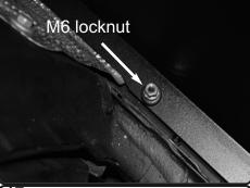
**17.** Secure and tighten the bottom of the heat-shield using provided M6 lock nut. Secure and tighten using 10mm socket or wrench.
