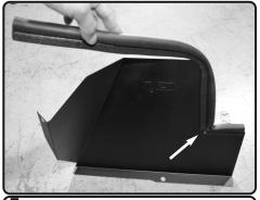
7. Install rubber trim to the top of the heatshield. Notch corner for easier installation.
