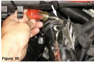
Once the intake has been aligned, continue to tighten the air duct clamp.
