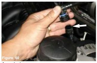
**Important:** The vacuum brake line is realigned as shown above. Vacuum line must be connected prior to starting engine.
