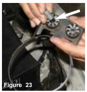
The aluminum stud is removed from one of the grommets.
