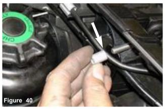
The 3/16" aluminum spacer is slipped over the m6 x 35mm bolt used to secure the reservoir bracket. **NOTE: Spacer is only required on the 135i**
