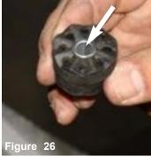
The aluminum stud is installed in the the stock grommet.
