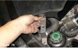
An m6 x 10mm bolt is used to attach the upper bracket to the second nut insert located on the air scoop.
