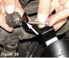
The 35mm bolt is inserted into the bent bracket attached to the cup and into the stock grommet.
