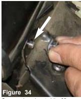
Once you have inserted the 35mm bolt all the way in, continue to place the m6 flange nut over the bolt end.
