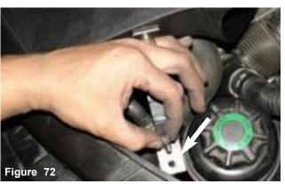
The second m6 x 10mm bolt is used to secure the lower bracket to the upper power steering reservoir bracket.
