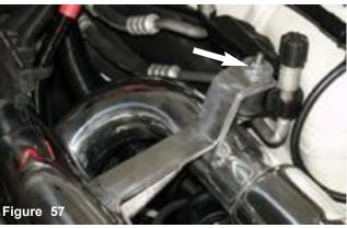
The m6 flange nut and fender washer is used to fasten the secondary intake to the vibra-mount stud.
