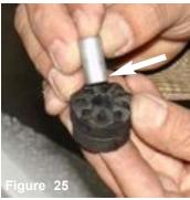
The aluminum stud in pressed into the grommet.
