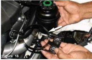
Once you have removed the m6 bolt, continue to remove the clamp from the power steering reservoir bottle.
