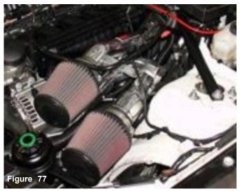
Over view of how the assembled filters and intakes should look like after its been installed and adjusted.
