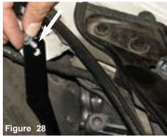
The stock m6 bolt is screwed into the pre-tapped hole.
