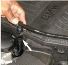
The hard plumbing vacuum line is detached from the lower hard line.
