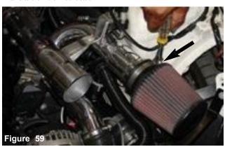
Once the intake end has butted up against the filter stops, continue to tighten the filter clamp.
