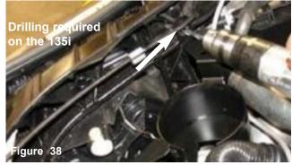
Applicable to the 135i only: Use a 1/4" drill bit to drill a hole through the composite cross member, the short bracket on the cup is used as a pattern.
