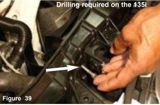
Insert the m6 x 35mm hex bolt through the composite cross member and through the 3/8" aluminum coupler as shown in figure 26.
