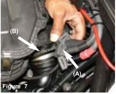
The harness rubber hangers have been removed from the prongs on the air box inlet(A). The inlet on the air box has also been separated (B).
