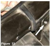
The 35mm bolt is inserted all the way through front of the cross member where the head lamp is fastened.
