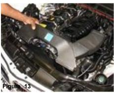
Once all four bolts have been removed, continue to pull the air scoop duct out.
