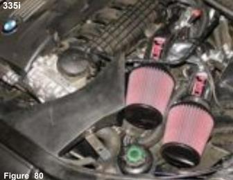
Congratulations! You have just completed the installation of this intake system. Periodically, check the alignment of the intake, normal wear and tear can cause nuts and bolts to come loose. Failure to check the alignment and adjust the intake can cause damage that will void the warranty.
