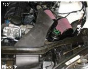
Align the entire intake for best possible fit. Once you have aligned and made sure that the length of the intake is free from any moving parts, continue to tighten all nuts, bolts and clamps.
