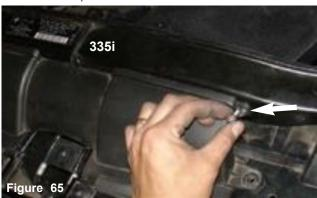
Attaching the air scoop to the 335i: The front scoop is re-attached to the cross member and the stock bolt is used to fasten the front scoop to the new engine air scoop. The plastic clips are also used on the scoop.
