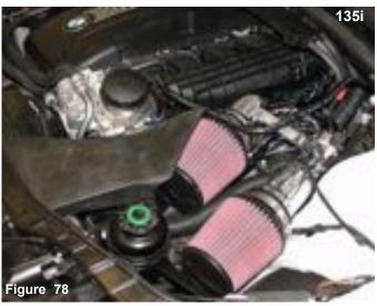
Note: The secondary filter on the 135i will fit snug inside of the air scoop as shown above. The secondary filter will have space around the filter when installed in the 335i.
