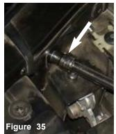
Use an m10 socket to tighten the m6 flange nut.
