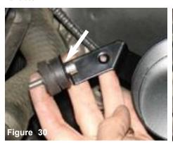
The 35mm bolt is inserted into the bracket and stock grommet.
