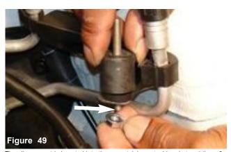
The vibra-mount is inserted into the new stainless steel bracket and the m6 flange nut is aligned to the vibra-mount stud.
