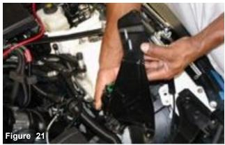
Once you have removed all nuts and bolts, continue to pull the power steering brace out of the engine compartment.
