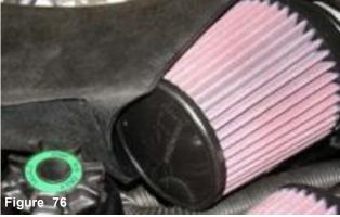
The second filter is now pressed over the secondary intake and adjusted in the air scoop. Once you have adjusted the filter, the intake clamp and filter clamps are tightened.
