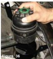
Once you have installed the reservoir cup in place, continue to lower the power-steering bottle in place.
