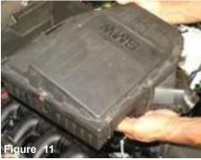
The air box cleaner is now ready to be pulled out of the engine compartment.
