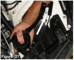
The reservoir cup is lowered into the engine compartment. The long cup bracket is aligned to the fender wall brace.
