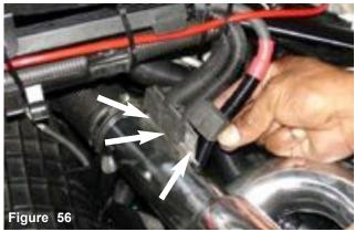
The three rubber harness hangers are pressed over the aluminum prongs located on the air intake as shown above.
