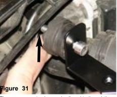
The new power steering cup is aligned to the existing bolt patterns. The 35mm bolts is screwed into the back side of the head lamp pre-tapped hole.
