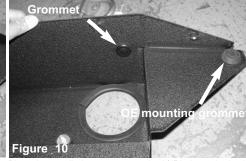
Place the supplied grommet onto the 3/4" hole on the back grommet for the 7/8" hole on the right side of the lower air
