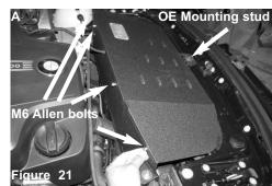
onto the back side of the air box cover to attach the air box cover to the lower air box.
