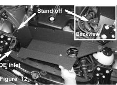
ing bracket behind the lower air box mounts on top of the stand off from figure 11. Also make sure the left side of the air box goes underneath the OE air box inlet.
