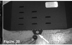
Place the second OE mounting grommet onto the end of the air box cover.
