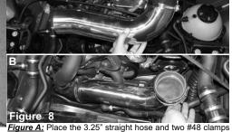
onto the end of the intake pipe and only secure the lower clamp for now. Figure B: Place the Injen intake pipe into the lower turbo inlet duct from figure 6 and leave the clamp loose for now. This pipe will need to be adjusted later.
