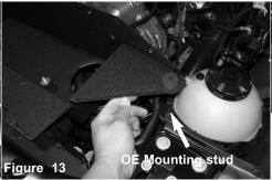
Place the supplied Stand off onto the left side OE air box Lower the lower air box into position. Place the left mount- Firmly push the right side of the lower air box grommet onto the OE air box mounting stud.
