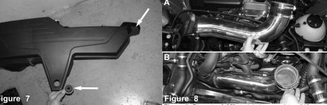
Remove the two factory mounting grommets from the OE air box assembly. These two grommets will be re-used later in the Inien intake kit.
