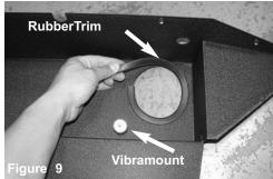
Place the Rubber trim around the 4" hole. Also screw the supplied Vibramount onto threaded hole next to the 4" hole of the lower air box and then re-use the OE mounting on the lower air box
