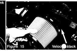
Depending on chassis and engine type, you may require Place the supplied filter onto the velocity stack to remove the tab on the coolant expansion tank. Firmly slide tab to the right and it will detach from the expansion tank. This tab might interfere with the heatshield cover.
