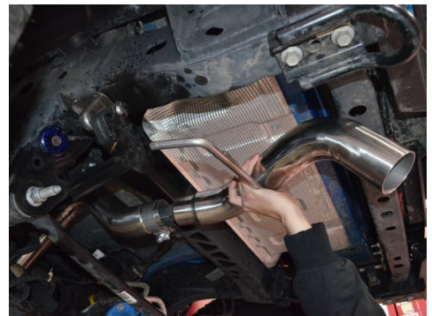
9. Insert the hanger to the rubber insulator then connect the muffler delete pipe to the mid pipe.
