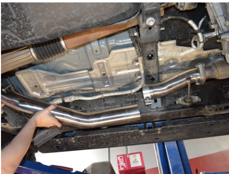
7. Connect the mid pipe to the front pipe. Secure using the provided 76mm clamps.
