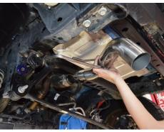
2. Insert the hanger to the rubber insulator then connect the muffler delete pipe to the mid pipe.
