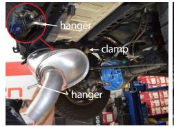
1. Remove the stock muffler by loosening the mid pipe clamp and detaching the muffler from the rubber insulators.
