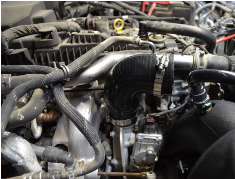
16. Install the 2.00"-2.75" elbow hose onto the turbo outlet. Only secure the clamp on the 2.00" side.
