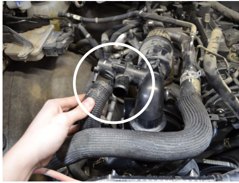
2. Release the tension clamp on the diverter valve outlet hose then detach the diverter valve hose.
