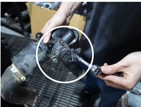
22. Remove the three bolts securing the diverter valve, then remove the diverter valve.
