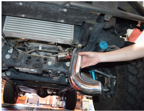
38. Install the cold side intercooler pipe. Insert the pipe into the bottom hose first, then into the top hose.
