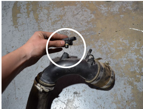
41. Remove the pressure sensor from the OEM cold side intercooler pipe.
