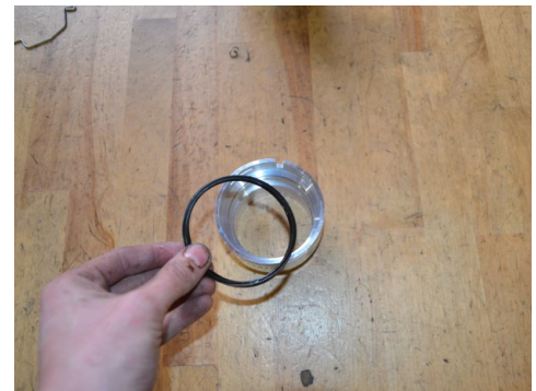
33. Install the OEM O-Ring onto the intercooler adapter in the same direction it was removed.
