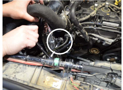
18. Secure the bracket on the intercooler pipe with the OEM bolt.
