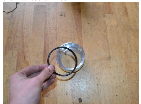
12. Install the OEM O-Ring onto the intercooler adapter in the same direction it was removed.
