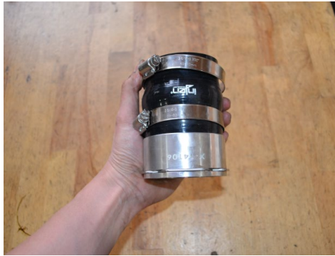
14. Install the 2.75" hump hose onto the intercooler adapter. Only secure the clamp on the adapter side.
