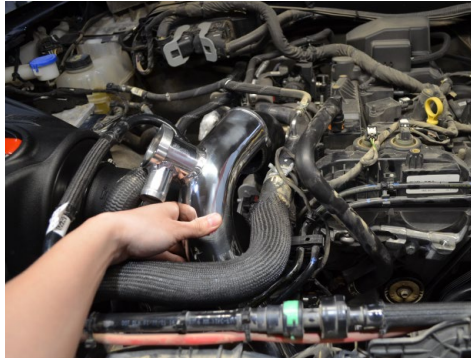
17. Install the injen hot side intercooler pipe. Insert the pipe into the bottom hose first, then into the elbow hose.
