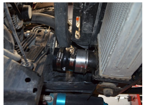
36. Install the intercooler adapter onto the intercooler outlet. A clicking sound will confirm it is properly secured.
