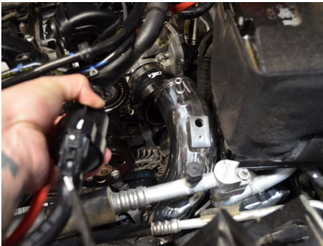
40. Once in position, secure all clamps on the top 2.75" hump hose.
