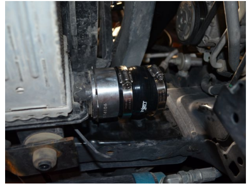
15. Install the intercooler adapter onto the intercooler inlet. A clicking sound will confirm it is properly secured.
