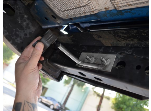
6. 2.3L MODELS ONLY: Insert the rubber insulator onto the exhaust hanger bracket.
