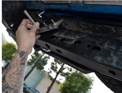
5. 2.3L MODELS ONLY: Slide the injen hanger bracket into place. Then secure the two bolts.
