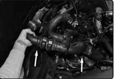
**11.** Now carefully lift up and remove the intercooler pipe out of vehicle.
