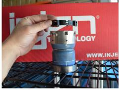
4. Remove the plastic retaining clip from the hot side turbo outlet coupler by carefully prying on both ends and then lifting up.
