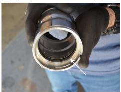
7. Install the provided O-Ring onto the secondary hot side intercooler pipe.
