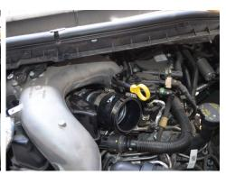
9. Install the 3.00" hump hose onto the Secure using the provided clamps.
