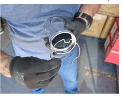
6. Install the OEM retaining clip onto the Injen secondary hot side intercooler pipe.
