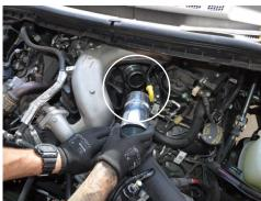
8. Install the secondary hot side intercooler pipe onto the turbo outlet. You secondary hot side intercooler pipe. should hear the retaining clip engage.
