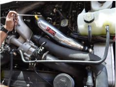
11. Install the Injen primary hot side intercooler pipe. Secure all clamps. Ensure the rtaining clip is properly engaged.
