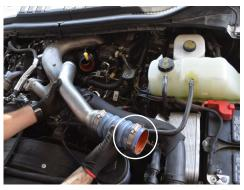
2. Loosen the clamp holding the hot side hot side intercooler pipe to the turbo inlet. intercooler pipe to the intercooler then remove the hot side charge pipe.
