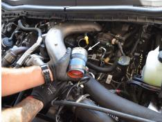
3. Disengage the retaining clip attached to the turbo outlet by prying up on the retaining clip then remove the hot side turbo outlet coupler.
