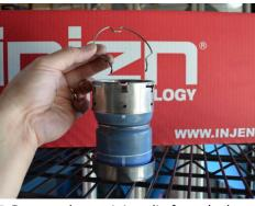
5. Remove the retaining clip from the hot side turbo outlet coupler.
