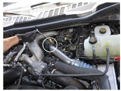
1. Loosen the clamp connecting the OEM
