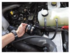
10. Install the 3.00" hump hose onto the intercooler. Secure using the provided clamps.
