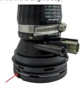
8. Remove the OEM retaing clip from the IAT sensor adapter.
