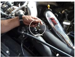
2. Lift the tab on the IAT sensor then twist 3. Loosen both clamps from the cold side the sensor a 1/4 turn to remove it from the intercooler pipe. cold side intercooler pipe.
