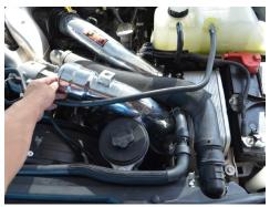
12. Once the intercooler pipe is in place. Secure the clampsthen secure the power steering reservoir to its factory location.
