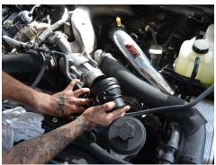
5. Disengage the retaining clip from the IAT sensor adapter then remove the adapter from the engine bay.
