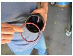
6. Remove the O-Ring from the IAT sensor adpater. Note the direction it was removed in.
