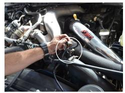
1. Disconnect the IAT sensor harness located on the OEM cold side intercooler pipe.
