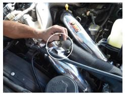
13. Install the IAT sensor onto the cold side 14. Reconnect the IAT sensor harness. intercooler pipe. Once fully seated, rotate the sensor to secure the tab in place.
