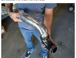
10. Install the elbow hose onto the cold side intercooler pipe. Secure using the provided clamps.
