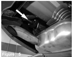
With lubrication, remove all the exhaust hangars from the rubber isolation mounts
