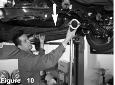
Now install the mid-pipe to the exhaust. Secure using provided 3" gasket and bolts with nuts.
