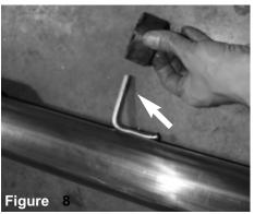
Remove the isolation mount from the exhaust closest to the 3 hole flange. Re-install to the new engine exhaust for easier installation.
