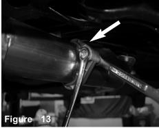
Install the last of the gasket with bolts with nuts. Position for best fit and clearance. Secure and tighten.
