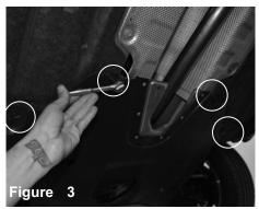
Loosen the screws holding in the factory engine cover. This will allow to loosen screws on pipe.
