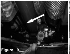
With provided 3 hole gasket, Install the front pipe to the 3 hole flange. Secure using original nuts from step 4.
