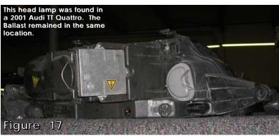
Late models such as this one has the HID ballast built into the head lamp.
