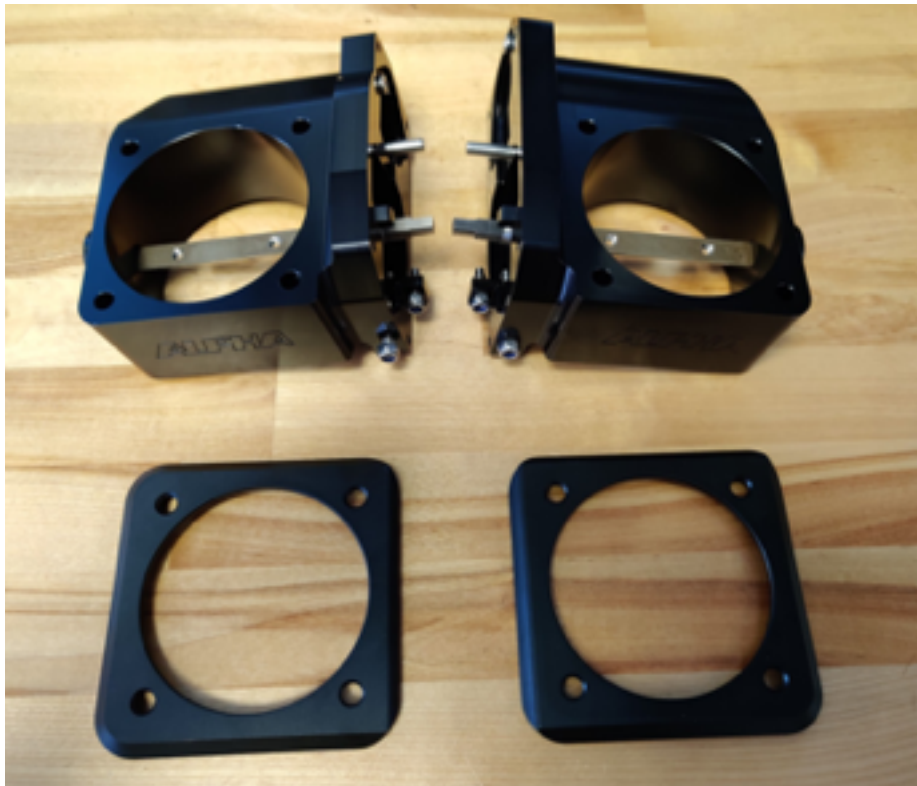
Figure 4: Gasket retainers shown beneath corresponding throttle bodies
