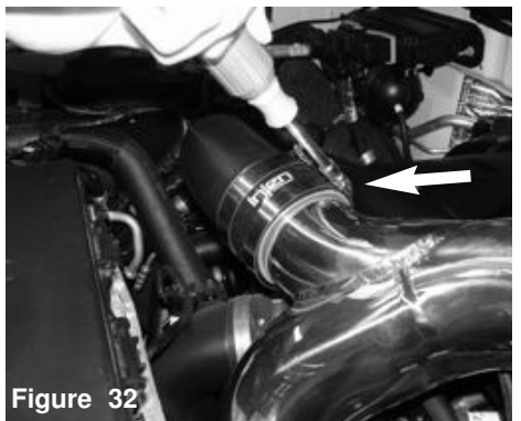
Figure 29 Install the hump hose with clamps to the larger side of the stock turbo inlet tube, Do not tighten.
