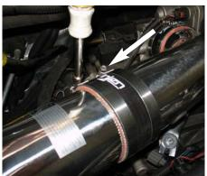
Position the intake for the best possible fit and clearance. Tighten all clamps using 8mm nut driver.
