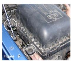
The grommets to the side of the air box cleaner is attached to the two pins on the air box brace. Gently, lift and pull the air box cleaner from the pins.
