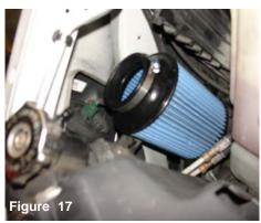
Position so it is easy to access the clamp when tightening to the intake tube. *Re-install the coolant bottle* for the remaining installation steps.
