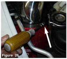
Instal the lower intake assembly and attach the filter to the tube. Tighen using 8mm nut driver. **Note:** may require an extra set of hands.
