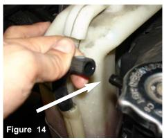
Pull back the coolant resovoir line, **NOTE:** make sure the vehicle is cool.
