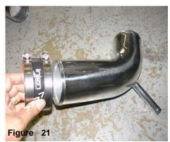
Attach the other 3-1/2" straight hose with clamps to the end of the upper intake assembly.
