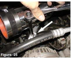
Tighten the upper intake assembly using 10mm socket and extension.
