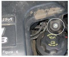
The second m8 bolt is removed from the air intake resonator located just above the oil cap.
