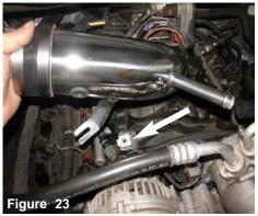
Install the upper intake assembly into the vehicle and position to thottle body and bracket to the engine
