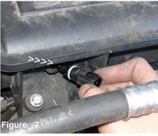
Turn the sensor 1/4 turn and gently pull the electrical air temp sensor from the air resonator grommet as shown above.
