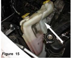
Loosen the 2 screws holding in the coolant resovoir bottle and lean back towards engine, this will allow for the filter installation.
