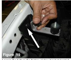
Loosen the bolt on the factory air box bracket located on the fender well using 13mm socket or wrench. install the new bracket and secure using the factory screw.
