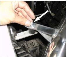
Secure the bracket to the vibra mount using M6 washer and nut.
