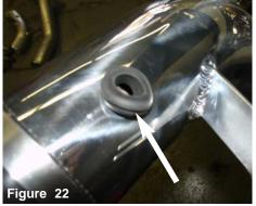
Attach the grommet to the hole cut out on the upper intake assembly tube, this will be used for the temperature sensor.
