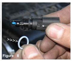
Remove the O-ring from the air temp sensor and set aside for now.
