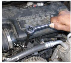
Loosen and remove the two front bolts that secures the intake resonator to the intake manifold.
