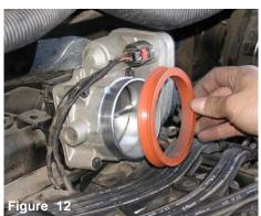
Remove the sealing ring from the throttle body as shown above.
