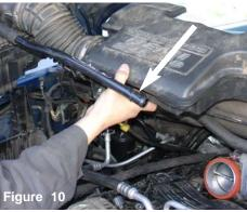
Once the air box has been lifted, continue to disconnect the crank case breather hose. **Late model trucks** has the breather hose connected to the air resonator.
