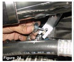
Install the M6 hex screw with flat washer and secure to the factory air box insert on engine.
