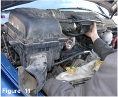
Lift and pull the air intake resonator from the throttle body. Once the air resonator has been disconnected from the throttle body, pull the entire air box out.
