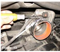
Press the new straight hose over the throttle body and use two power-bands. Tighten the power-band located over the throttle body for now.
