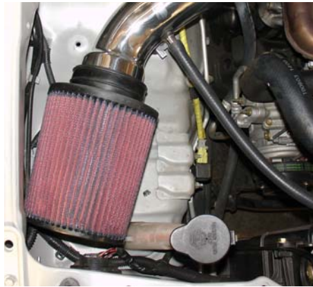
Once the filter has been placed over the intake end and the intake is set up against the filter stop continue to tighten the filter clamp.
