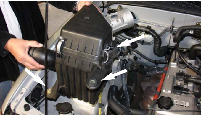
Remove the m6 bolts holding the air intake box to the fender well. Remove the vacuum hose connected to the air box. Pull the air intake box out of the engine compartment.
