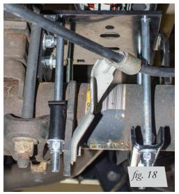
Right side (passenger) forward axle view of finished installation torqued to 10 lb.-ft. (14Nm).
