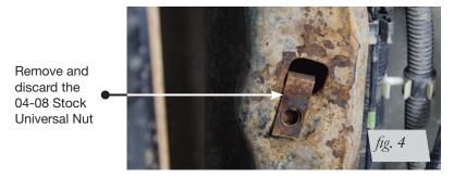
4. For the early 04-08 models, install a new universal nut (V) into the large hole so that the threaded portion is up inside the frame (Fig. 5).
