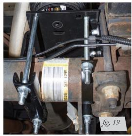
Right side (passenger) rearward axle view of finished installation torqued to 10 lb.-ft. (14Nm).
