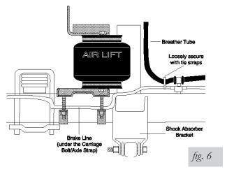
7. Using the holes in the upper bracket as a template, drill two 5/16" holes into the frame. Insert and tighten the self tapping bolts (K) and torque to 15 ft-lbs. (Figures 1 and 7).
