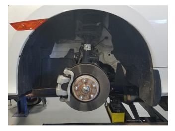
2. Remove stabilizer link nut from strut tab and stabilizer bar. Remove stabilizer link from vehicle.
