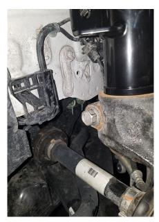
4. Pull the steering knuckle outward and insert the front driveshaft through the hub. Reinstall the front driveshaft spindle nut. Do not torque the nut at this time.
