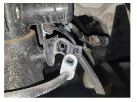
5. Remove the wheel speed sensor wire from the retainer on the strut.
