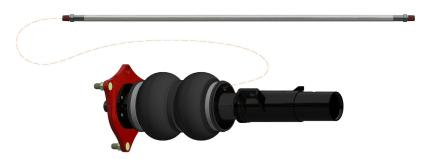
2. Insert the Air Lift Performance strut upper mount into the chassis and install the upper mount nuts. Ensure left-hand and right-hand struts are installed in the correct side. Torque the nuts to 75Nm (55 lb.-ft.).
