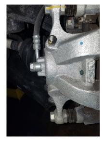
8. Reinstall the brake hose retaining bolt and torque it to 22Nm (16 lb.-ft.). Place the ABS sensor wire back into the retainer.
