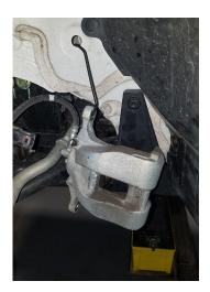
7. Use a punch to push out the staked section of the spindle nut shoulder. Remove the front driveshaft spindle nut.
