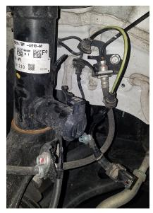
4. Remove the brake hose retaining bolt.
