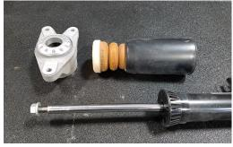
5. Install upper shock mount on Air Lift Performance shock with supplied nylon lock nut. Torque nut to 20Nm (15 lb.-ft.). Reinstall dust cap on upper shock mount.
