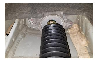
7. Raise lower control arm and install lower shock mount bolt. Do not torque bolt at this time. Reinstall ABS sensor wire on shock tab.
