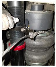
8. Install Air Lift Performance toe link with previously removed bolts and included spacers. Arrow on toe link should point toward wheel. Do not torque bolts at this time.
