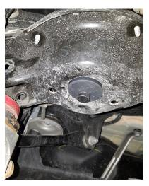
4. Remove dust cover from upper shock mount. Unbolt the upper shock mount from the shock rod. Separate the jounce bumper/dust cover from the upper mount.
