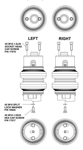
2. Air spring assemblies are side specific. Insert the correct air spring into the lower control arm. Align lower bracket with spring pocket in lower control arm.
