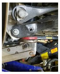
6. Remove upper shock mount bolts and remove shock from vehicle.
