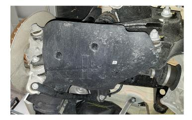
10. Before lowering vehicle on wheels upper air spring spacer should be seated. Install air line in air spring and slowly inflate to at least 3.5BAR (50PSI) while guiding upper mount pilot into chassis.
