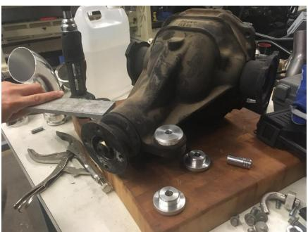
**Step 6:** Reinstall the differential: Use the supplied bolts for the front mounts of the differential. Front and rear differential bolts are to be torque to **72-87 ft-lbs** using a torque wrench. *Thread locker is recommended.*
