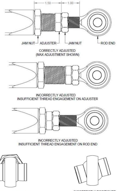
INCORRECTLY POSITIONED TOO MUCH STATIC ROD END MISALIGNMENT
