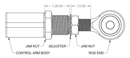
CORRECTLY ADJUSTED (MAX ADJUSTMENT SHOWN)
