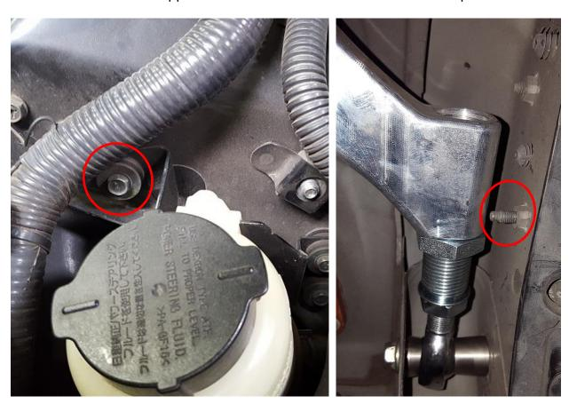
**Step 6:** Using a 10mm socket and ratchet (recommended to use 3/8" drive), adjust the front and rear adjusters to desired camber and/or caster settings. If factory caster is desired, adjust evenly. Using an 11/16" end wrench, tighten smaller rod end jam nuts against adjuster flange securely. Use 10mm socket again to align rod end position as shown on next page. Using a 1-1/4" end wrench, securely fasten the larger jam nut against the control arm body.
