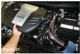
Reinstall the engine cover. Your intake installation is now complete. Go over all your clamps and fittings to make sure they are snug. Check the clearance on the pipe and make sure it does not make contact with any components in the engine bay.
