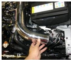
Line up the intake bracket to the vibra mount in figure
