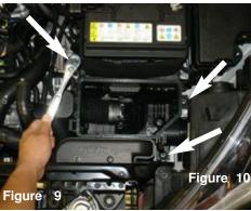
Use a 10mm socket, rachet and extension to remove the three 10mm bolts on the lower air box assembly indicated by the arrow.
