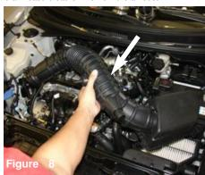
Remove the entire upper air box assembly and air duct from the engine bay
