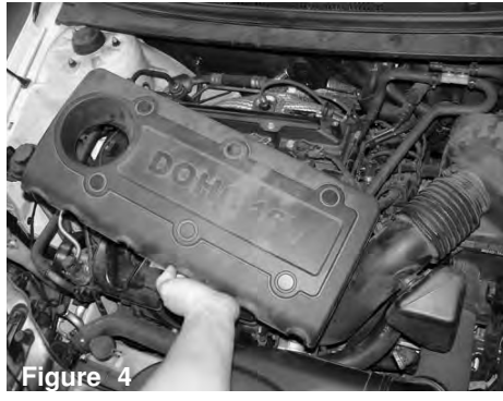
Figure 4 Remove the plastic engine cover by firmly lifting up.
