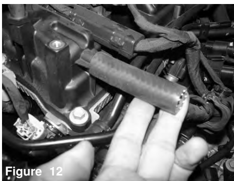
Figure 12 Attach the provided 12mm hose to the crank case fitting on engine.
