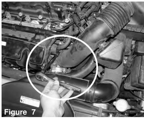
Figure 7 Use a 10mm socket and ratchet to loosen the clamp on the air duct connected to the throttle body
