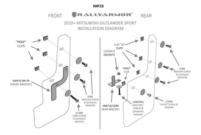
Check wheel clearance after installation, especially on vehicles outfitted with non-OEM offset wheels and suspensions. Adjust to accommodate accordingly in these scenarios. <u>Rally Armor is not responsible for damage or loss of installed flaps</u>.
