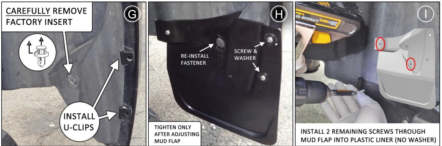
Figure I. – Using a Philips driver, install two screws (no washers) through the remaining mounting holes. The screws will self-tap and go into the plastic liner.
