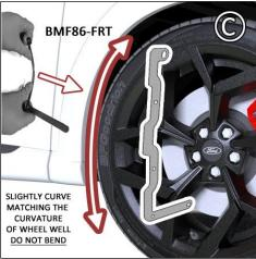
**FIGURE D** Position BMF86-FRT bracket behind mud flap. Stud facing forward, install HXBLT behind bracket, through flap on mounts 2 - 4. Install HXNUT & SMWASH on flap side. Do not fully tighten.
