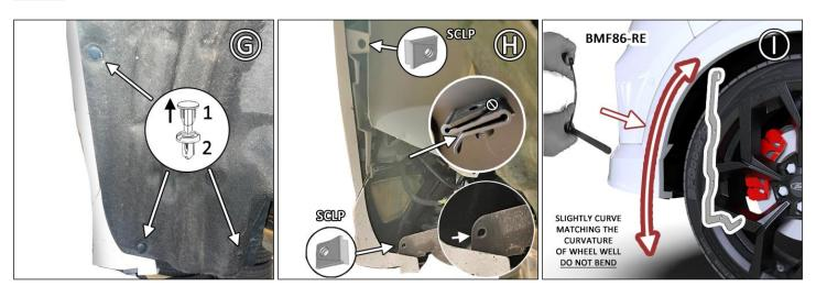
**FIGURE J** Position BMF86-RE bracket behind mud flap. Install HXBLT behind bracket, through mud flap, stud facing forward on mounts 2, 3 & 5. Install HXNUT & SMWASH on flap side. Do not fully tighten.
