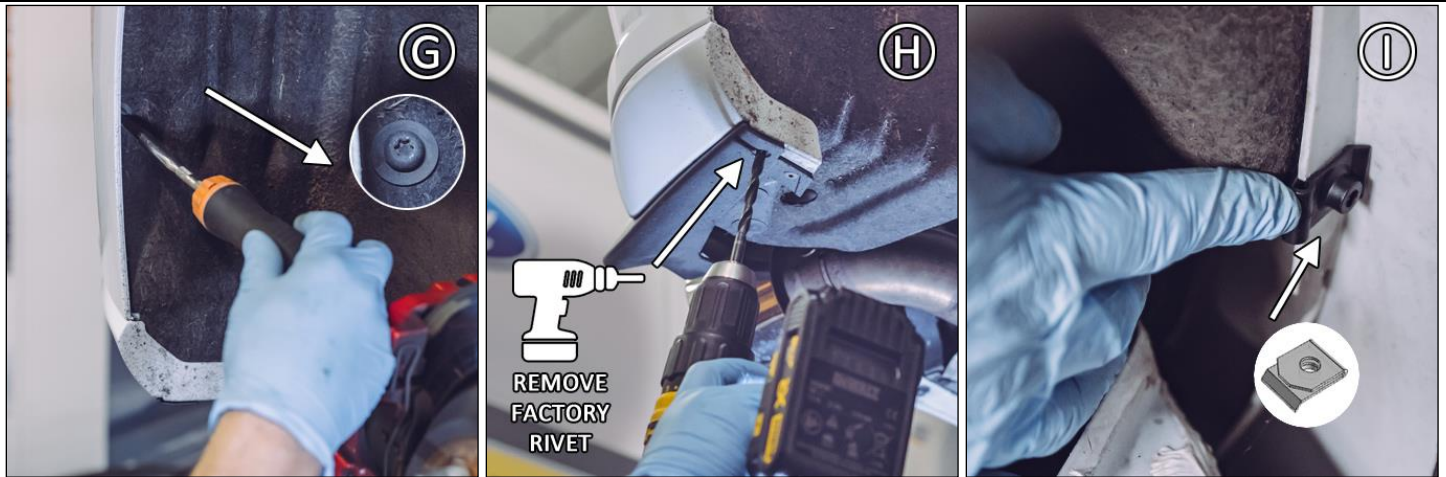
FIGURE J/K Install lower mounting point of rear bracket BMF77-LR/RR with 1MCHSS and SSLNUT.
