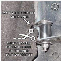
FIGURE M The upper portion of the bracket installs between bumper and liner. The lower bracket area requires adjustment by carefully curving the lower mount forward then backward until it seats and nests flap properly. Avoid overextending the bend.
