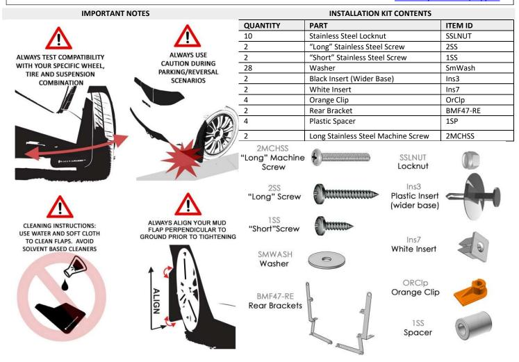
Recommended Tools Low-profile, ratcheting offset or stubby Phillips screwdriver, small flathead screwdriver, pick, 7/16" wrench, panel removal tool. Important Tips Installation should be done on an even surface. The hardware self-threads so avoid overtightening.
