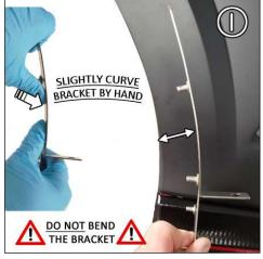
FIGURE J As shown in J, gently create a curve by pressing the bracket's innermost rear section close to the liner after it's installed. Do this gradually so you don't extend the curve beyond the liner. The intent is to fill the gap by bringing the part close to the liner.
