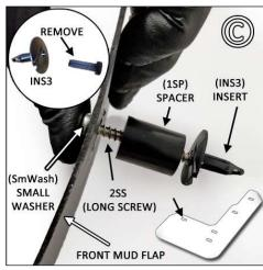
**FIGURE D** INS3 Insert assembly goes into mounting point 4. It should be firmly seated against the liner. Hold female base portion of insert securely against liner to prevent it from spinning. Continue threading the Long Screw (2SS), keeping the Insert seated against liner during this process. Tighten until washer is *almost* seated against the flap. Do not fully tighten so you can adjust later.
