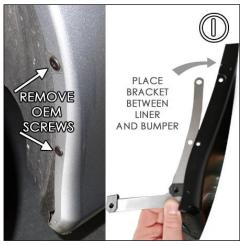
**FIGURE J** Install OEM screw and Small Washer through mud flap, bumper and mounting bracket 1 & 2. Install Short Screw 1SS in points 3 and 4. The lower section of the bracket should be parallel to the tire.
