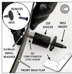
**FIGURE D** Insert 3 INS3 assembly goes into mounting point 4, firmly seated against the liner. Hold female base of insert securely against liner to prevent it from spinning. Continue threading the Long Stainless Steel Screw 2SS, keeping Insert 3 seated against liner during this process. Tighten until Small Washer is *almost* seated against the flap.
