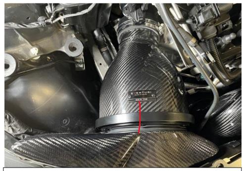
57. Once past the actuator it can be positioned onto the turbo inlet. Rotate the housing so that the Plaque lines up with the groove on the duct as shown.
