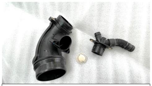
12. Remove the breather assembly from the inlet. There is also a metal shim inside the breather hole of the inlet.
