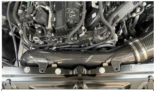
37. Remove the cloth and rotate the tube so that the carbon brackets sit flat on the slam panel.
