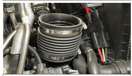
27. Position 2 x 80-100mm hose clamps as shown and tighten the lower one around the inlet. Do not over tighten.
