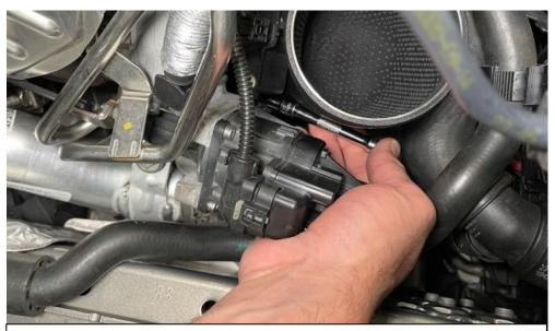
21. An example of how to turn the screw using an extension.
