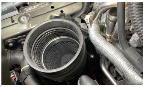
26. Push the hose onto the inlet making sure the TOP stays on top. Push it down fully so the inlet ends where the flexible portion starts.
