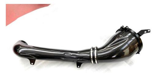
33. Assemble the carbon tube and RHS housing as shown using the supplied silicon hose and 2 x 100-120 clamps . The RHS housing has a bracket attached to the front and curves
