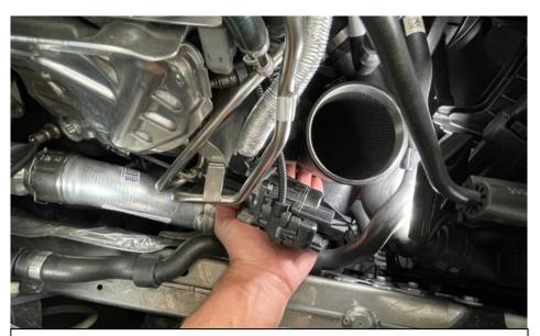
19b. The other side is more tricky to get to - you can reach under the turbo module as shown to support the screw on this side and get it into place.
