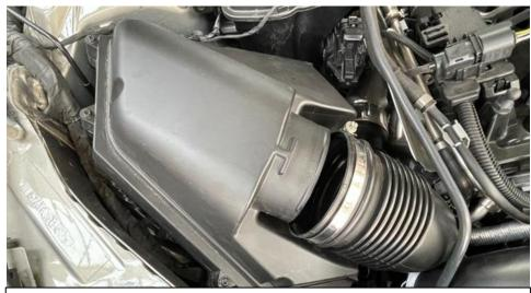
2. Starting with the left side (as you look at the engine from the front of the car) loosen and remove the flexible tube from the airbox. The Pull the airbox out - it is held in with rubber grommets.
