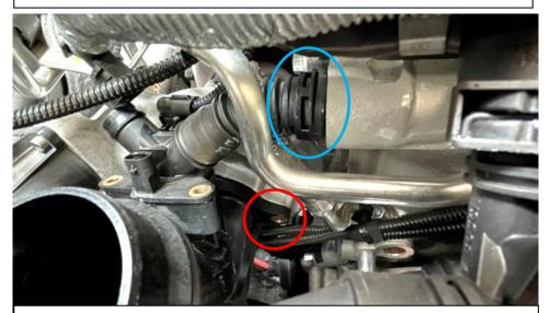
11. Inlet is held in place with 2 screws, one circled red and the other on the opposite side. Remove the screws. There is also a breather hose going into the engine (circled blue) - unclip from the engine side and you can pull this out as the inlet is removed.
