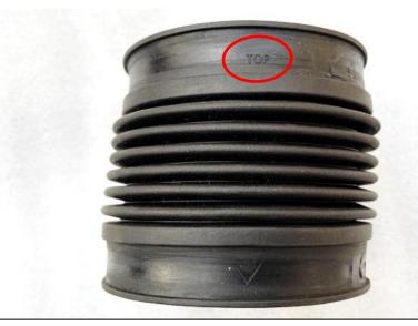
25. Take the new flexible rubber hose and identify the TOP as printed on the hose shown.
