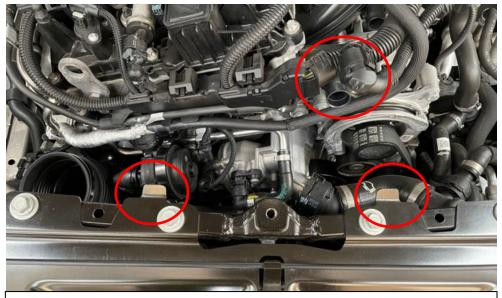
31. Before lowering the carbon tube int place - we need to cover the metal tabs shown and also make sure the plug removed previously is out of the way.
