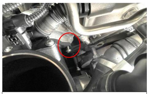
19. Line up the inlet and use one screw on the right side - turn it by hand to ensure you do not cross thread the turbo. DO NOT fully secure yet - leave it loose.
