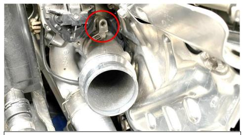
4. Remove the 2 screws holding the turbo inlet in place and pull the inlet out. One screw is circled and the other is on the opposite side hidden from view.
