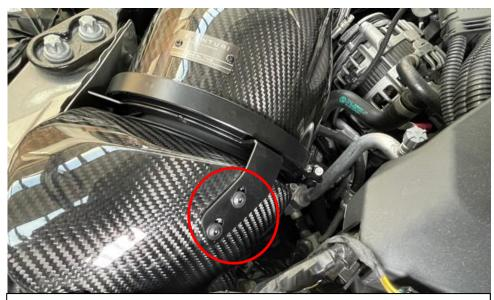
41. Using the supplied M5 screws - secure the bracket to the duct.
