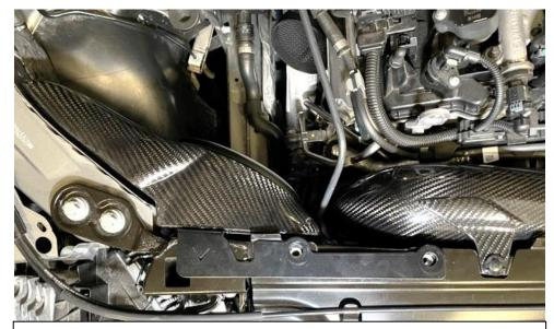
51. Position the duct so the bracket lines up with the 2 holes.
