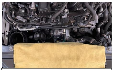
32. Cover the metal tabs with a cloth to protect the carbon tube.
