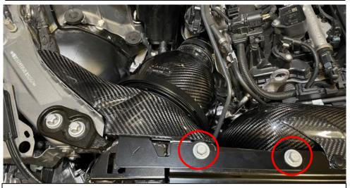
59. Insert the 2 x stock bolts previously removed and tighten.
