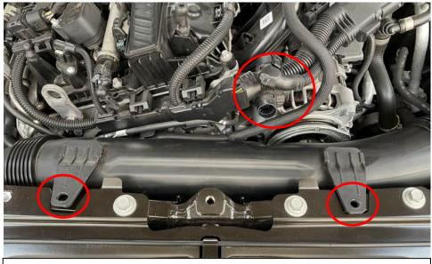
6. Unclip the plug shown to allow more clearance for the tube. Also remove the 2 plastic push clips in the tube brackets.
