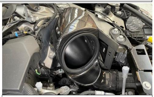
29. Lower the duct into place - it should connect to the OEM air duct as shown.
