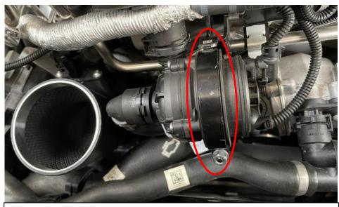
24. Secure the module from step 10 and re-attach the bracket with the 10mm nut.
