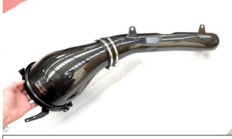
34. Another angle of the housing and tube. Leave the clamps loose to allow the housing to be rotated.
