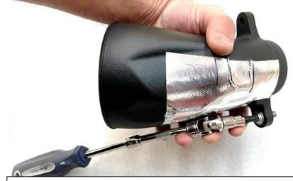
45. Accessing this screw with the inlet in place is tricky - we suggest to use a 1/4 " drive with a swivel socket located onto the screw as you lower it into place.
