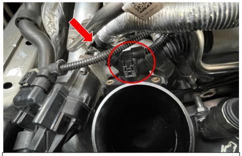
9. Remove the sensor plug on the turbo inlet and also the breather shown by the arrow. Breather is held in by a clip which can be squeezed to release.
