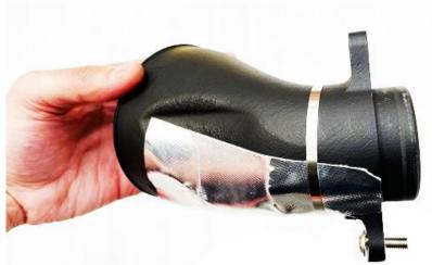
44. Take the LHS turbo inlet and push 1 x M6 Torx screw (provided) into the lower hole shown. There is also an O-ring inside the hole, make sure it stays inside.
