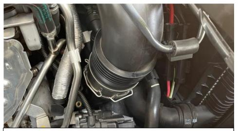
7. Pull out the retaining clip on the bottom of the intake tube to release it from the turbo inlet. Now pull the tube out.
