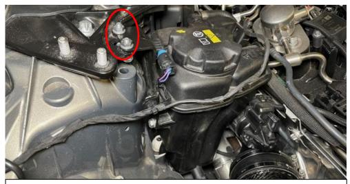
60. Locate the coolant tank back into position. Make sure it goes back into the white rubber grommet. Tighten the bracket with the 2 x 10mm nuts.
