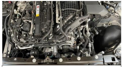
8. You can now remove the entire tube/airbox assembly from the car. The airbox pulls out.
