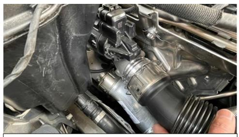
3. Pull out the retaining clip around the back of the tube and remove the tube from the metal turbo inlet.
