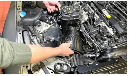
55. Lift the coolant tank and lower the LHS housing down.
