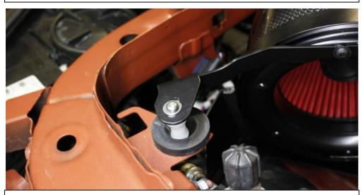
41. Locate the mounting boss over the stock rubber grommet. If required, rotate the mount and filter assembly in the housing. Band clamp should be loose enough to allow this – otherwise loosen to allow rotation. (Photo shown without the duct)
