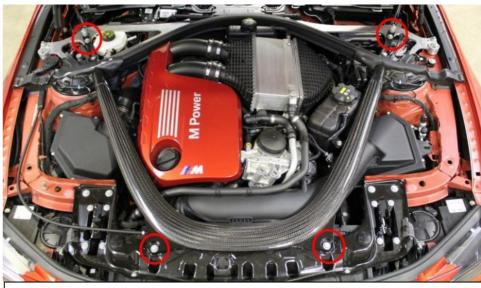
2. Remove the 8 13mm bolts holding the strut brace down. There is also a 10mm bolt secured to the coolant tank – see next photo.
