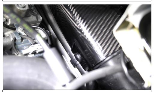
23. Starting on the side closest to the engine - align the hole on the new duct with the hole on the stock opening and push the rivet through. Secure by clicking the head in fully.
