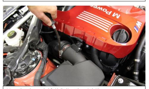
4. Loosen hose clamp on the left side (looking at the engine) airbox.
