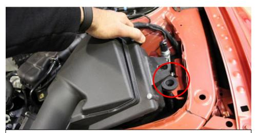
15. Pull the right side of the airbox upwards and out of the rubber grommet as can be seen here. Remove the airbox and tube assembly completely from the engine bay.
