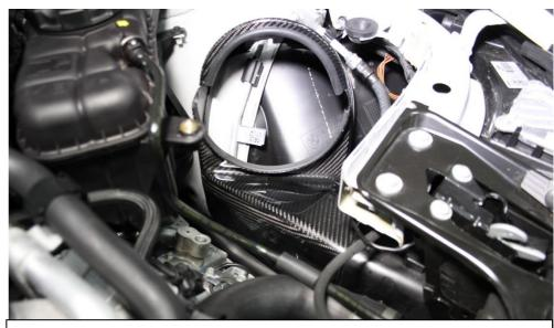
21. Take the right side duct (larger one) and locate the holes at the back over the holes shown previously on the stock duct opening. The new duct should go OVER the stock one.
