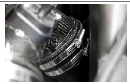
34. Push the tube all the way into the silicon so that the flange on the tube meets the silicon all the way around. Don't tighten yet.
