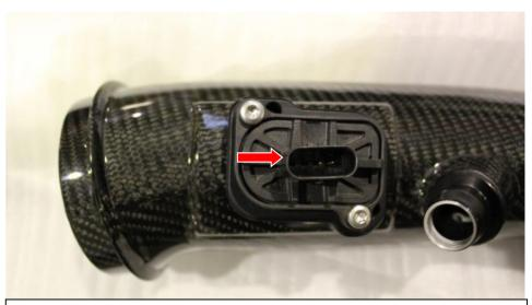
18. Insert MAF sensor into RHS tube – **ensure that the sensor is oriented correctly**. There is an arrow on the sensor indicating direction of airflow which is highlighted here in red. Secure both sensors with the supplied M4 torx screws.
