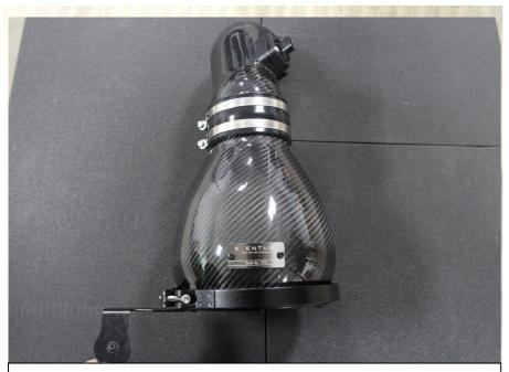
32. Orient the tube as shown. Tighten Hose clamp on the housing, leave the clamp on the tube loose enough to allow the tube to still be rotated.
