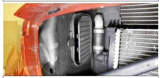
49. Here you can see the font of the grid has been released and can now be removed. Do the same for the other side.
