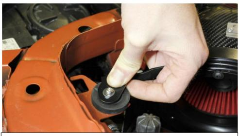
42. Push the mount all the way into the grommet. (Photo shown without the duct)
