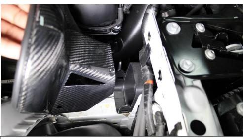
25. Looking at the other side – identify the 2 holes on the stock opening which will again be used for location and securing the left side duct.
