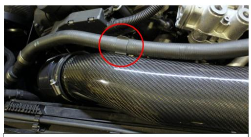
39. Push the stock rubber hose into the metal clip on the carbon tube.
