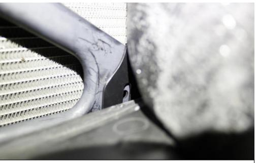
61. As previously, align the bracket with the hole on the strut brace and secure with the push rivet.
