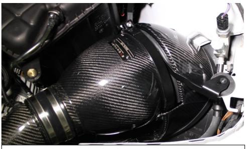
40. Place the mouth of the intake into the duct.
