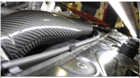
44. Rotate the carbon tube to allow a gap over the fan shroud. The hose clamps on either side of this tube should still be loose to allow rotation.
