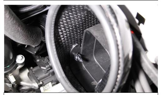
27. Use the 2 push rivets to again secure the duct in place. Press the rivet heads in fully to lock. Again, there will be some movement in the duct - which is required.
