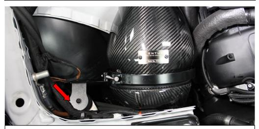
35. Push the boss on the mounting bracket into the stock rubber grommet fully. Ensure the housing is positioned evenly into the seal of the duct.
