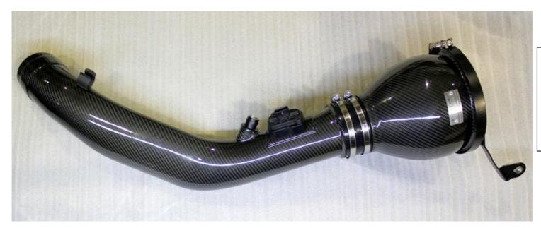
37. Assemble the right side intake with the long carbon tube as shown using the remaining silicon coupler and hose clamps. When pushing the silicon coupler onto the housing **DO NOT PUSH ON THE FILTER ITSELF.** Tighten the clamp on the housing, leave the clamp on the tube loose to allow it to rotate.
