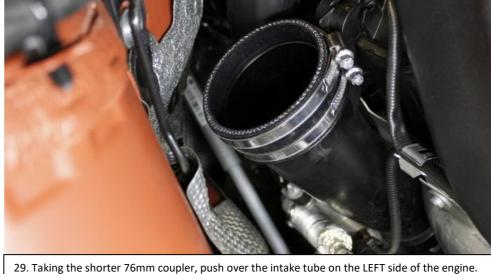
29. Taking the shorter 76mm coupler, push over the intake tube on the LEFT side of the engine Make sure the coupler is pushed down fully and put two hose clamps around the coupler as shown. Tighten the LOWER clamp only.
