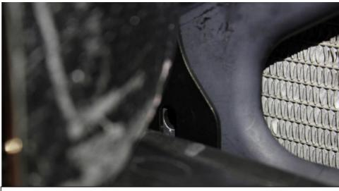
54. The bracket should line up with the hole in the strut brace as shown.
