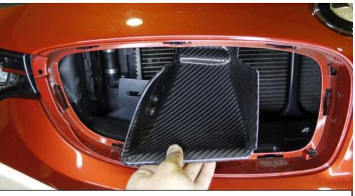
51. Insert the LHS scoop into the left side as shown with the bracket towards the left headlight. Once inside, rotate 90 degrees counter clockwise so that the bracket faces down. The scoop should be positioned as shown in the next steps.
