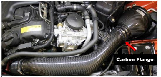
46. Once positioned correctly, tighten the hose clamps on both sides of the carbon tube. Ensure there is no gap between the flange on the carbon and the silicon as shown. Reinstall strut brace with all 13mm bolts and the 10mm bolt.
