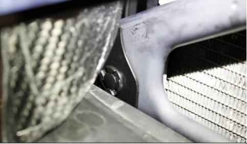
56. Push rivet fully secured in place.
