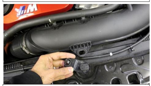
12. Remove the centre mount from the tube by pushing the two tabs together and down.
