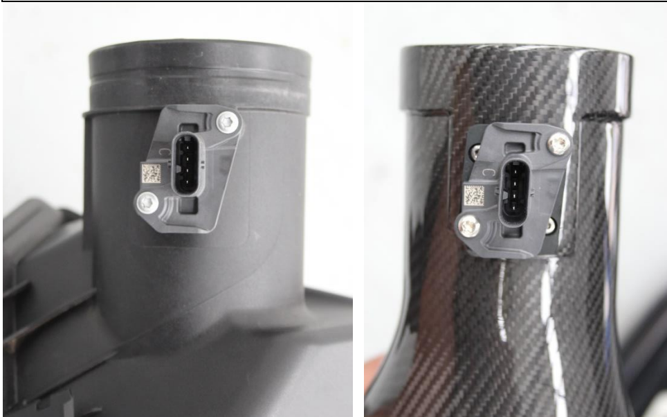
7. Remove the MAF Sensor from the stock airbox and install into the carbon housing using the supplied M4 screws. DO NOT USE THE STOCK SCREWS.
