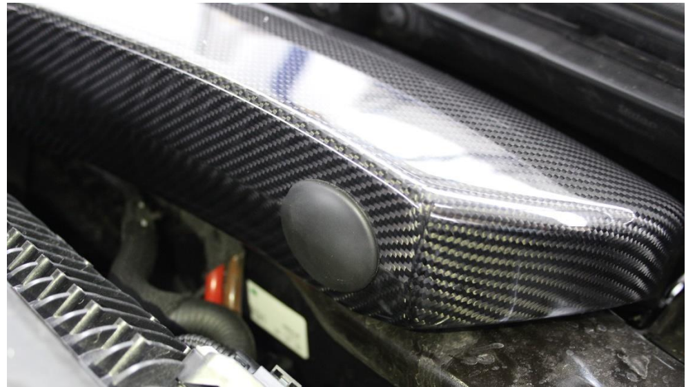
12. Close the Access Hole with the supplied rubber plug.
