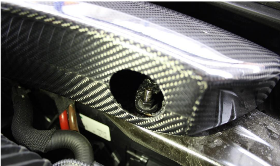
11. Secure the left side by using the stock nut through the access hole as shown.
