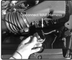
**3.** Disconnect the MAF sensor harness and remove line away from the airbox.
