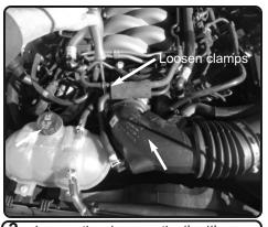
**2.** Loosen the clamp on the throttle body using 7mm nut driver or flat head screwsdriver.
