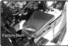
11. Drop the Injen lower air box assembly into the factory air box location. The front ram air should just slide into the Injen air box.
