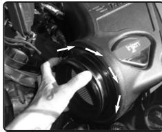
**4.** Once seated, Secure the twist lock filter by rotating in either direction 1/4" turn untill filter locks into place.
