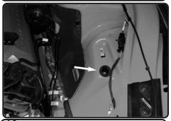
**10.** Install the larger grommet from figure 8 and install it into the original hole location on the fender well.
