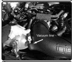
**9.** Re-connect the vacuum line to the 3/8" fitting.
