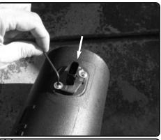
**14.** Now install the MAF sensor into the new injen intake tube using provided M4 screws and secure.
