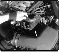
**6.** Disconnect the sound tube resonator box from the air box.
