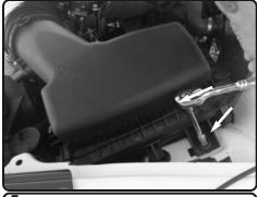
**5.** Remove the 10mm bolt from the OE air box assembly.
