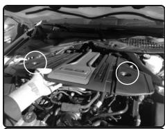
1. Stock intake system shown. Loosen the 2 nuts holding in the engine cover. Remove engine cover.
