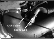
**10.** Re-connect the crank case line to the 5/8" fitting. Re-connect the sound tube and secure.
