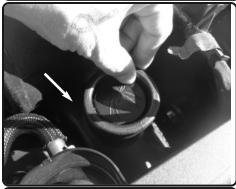
**5.** Install the provided filter monitor plug into the slot. ( Sold seperately is our injen filter monitor see injen.com for more info)
