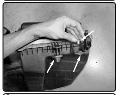
**8.** Remove the two grommets and spacer washer from the OE air box assembly
