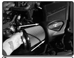
**3.** Install the twist lock filter into the air box. Install the provided 4mm vinyl to the fitting on the top of the air filter. ( if not using injen filter monitor)
