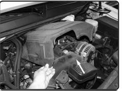
**2.** Pull the engine cover off the intake manifold.
