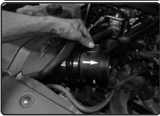
**22.** Install the MAF sensor to the hump hose. *Make sure Arrow on sensor is going in direction towards the throttle body.*
