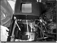
**19.** Now install the air box assembly into the vehicle. Position the tabs to seat like OEM box.
