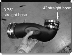
**18.** Install the the 4" and 3.75" straight hoses to the tube with clamps provided.
