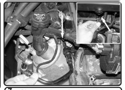
**7.** Disconnect the crank case ventilation line from the air duct resonator section located on top of the intake manifold. You will need to unclip a plastic lock in order for you to remove this line from the valve cover.
