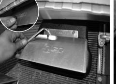
Install the rain guard. Secure using provided M6 socket cap screws and tighten. Once secure, cover the socket cap screw using provided vinyl cap. This will prevent any contact with screws and front bumper support. Failure to do so will result in vibration noise.
