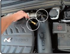
**16.** Reinstall the factory vacuum lines onto the fittings located on the Injen intke
