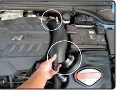
**15.** Place the Injen intake tube into the 3.50" hose end and the other end of the tube into the filter inlet.
