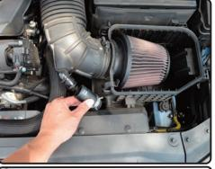
**2.** Detach the diverter valve return line from the stock intake tube
