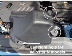
**10.** Place the three grommets from figure 9 onto the Injen air box. *Note:* Confirm grommet location on the Veloster N models in the photo.
