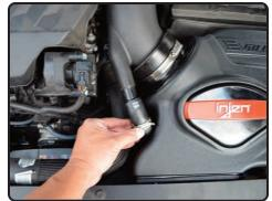
**17.** Reattach the diverter valve return line to the Injen Intake tube diverter valve port.
