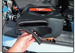
**11.** Install the 18" bulb trim onto the Injen air box inlet.
