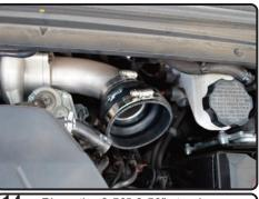
**14.** Place the 2.50"-3.50" step hose, #36 and #56 clamp onto the turbo inlet. Secure only the 2.50" hose end to the turbo inlet using the #36 clamp for now
