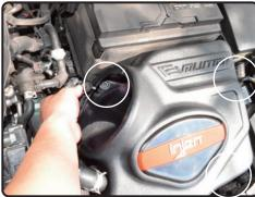
**12.** Lower the Injen air box into the engine bay and secure it using the 3 original 10mm bolts
