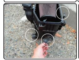
**9.** Remove the three grommets and spacers from the stock air box assembly. Grommets will be reused on the Injen air box
