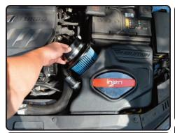
**13.** Place the Injen Twist Lock filter into the Injen air box. Make sure you rotate the filter until you feel it engage
