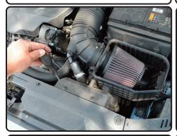
**5.** Press the two pins on the plastic rivets on top of the factory inlet scoop and then remove the rivets
