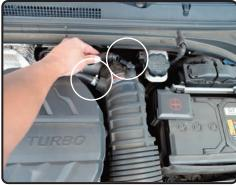
**3.** Disconnect the two vaccuum line on the stock intake tube
