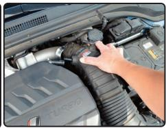
**4.** Loosen the clamp on the stock intake hose and disconnect the hose from the turbo inlet
