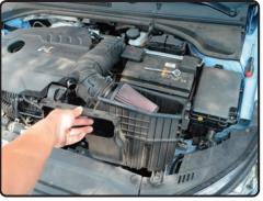
7. Lift the stock air box, intake tube and scoop assembly from the engine bay.
