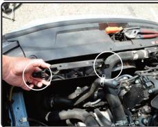
**8.** Remove the two screws from the front scoop bracket and then remove the scoop bracket.
