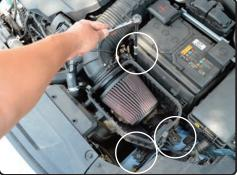
**6.** Remove the three 10mm bolts from the factory air box assembly
