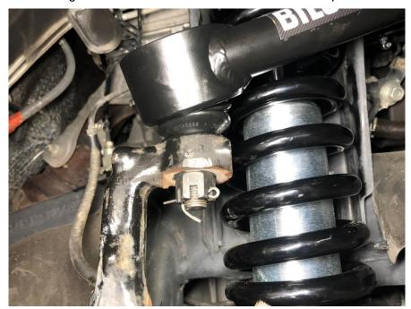
P. Reinstall the Sway bar link using a 17mm wrench. Reinstall the brake line bracket to the spindle using a 12mm wrench.
