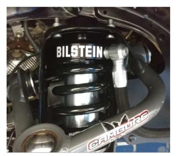
M. Attach the lower shock mount with the OE shock bolt and nut that was removed in Step A (1 per side). **Torque lower OE shock bolt and nut to service manual specification.**
