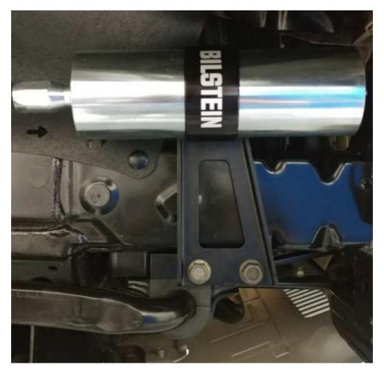
V. Re-attach and torque outer tie rod, control arm to knuckle ball joint nut, and sway bar link according to service manual specifications.
