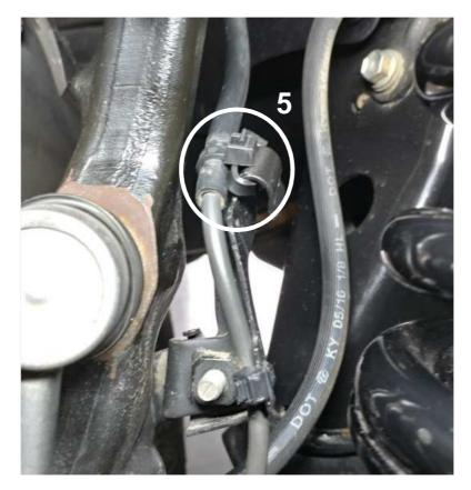
AA. Once the ABS line has been relocated as shown above, the installation is complete.
