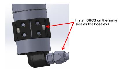
AA. Prepare the following assembly by applying non-permanent thread locker to two Flange Head Cap Screws (BOM item #6). Mount the Reservoir Clamp to the Reservoir Mount Plate (BOM item #11) as shown below using the two Flange Head Cap Screws. Tighten using a 13mm socket.
