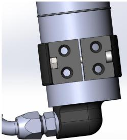
R. Prepare the following assembly by applying non-permanent thread locker to two Flange Head Cap Screws (BOM item #6). Mount the Reservoir Clamp to the Reservoir Mount Plate (BOM item #5) as shown below using the two Flange Head Cap Screws. Tighten using a 13mm socket.
